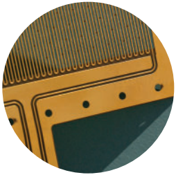
LDI imaged antenna – .004/.004 with perfect front to back registration.
